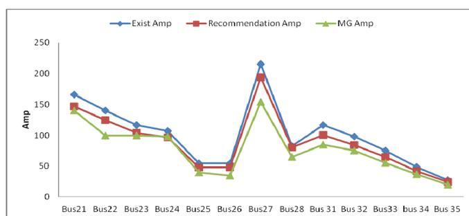
Fig. 15. Load Current Profile after MG Recommendation
