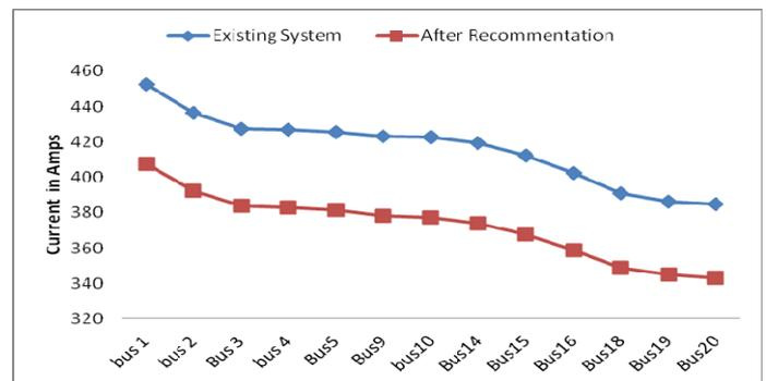
Fig. 13. Load Current Profile After Recommendation
