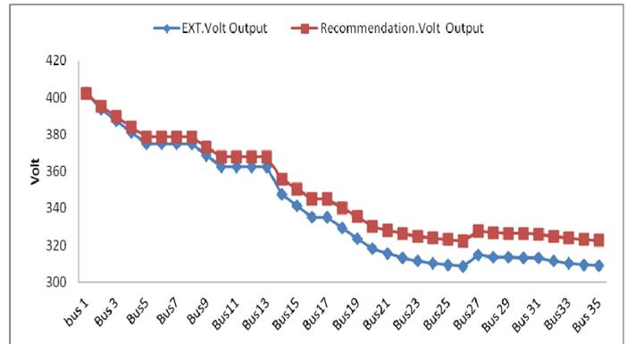
Fig. 12. Bus Volt. Profile After Recommendation
