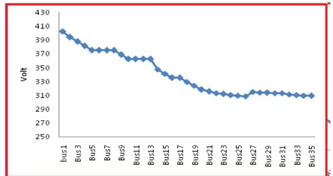
Fig. 3. Bus Voltage of Existing Test Feeder in ETAP
