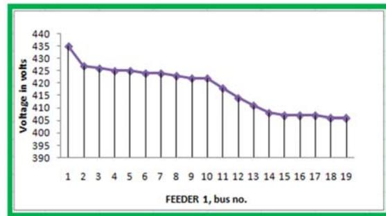
Figure-4 (a).Output voltage of existing system2 (Feeder1).
