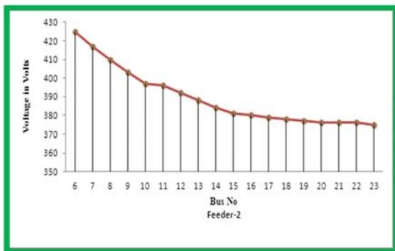
Figure-2(b).Output voltage of existing system1 (Feeder2).
