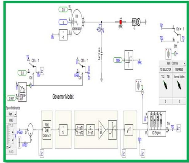
**Figure-6.** Modeling of diesel in PSCAD.
