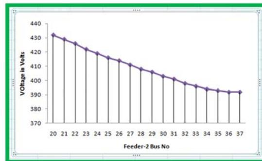
Figure-4 (b).Output voltage of existing system2 (Feeder2).
