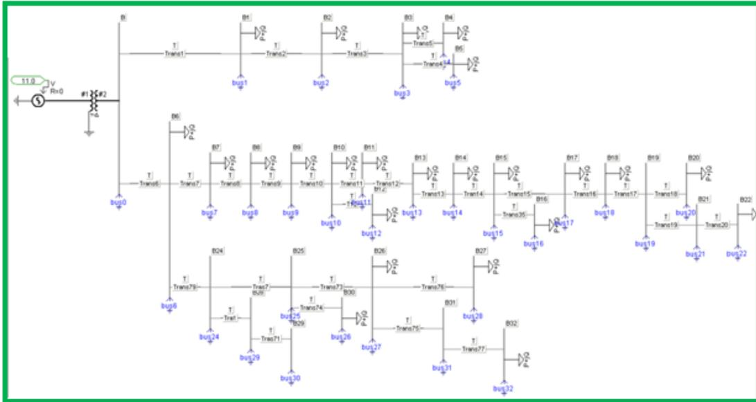
Figure-1. PSCAD implementation of existing system of region 1.
